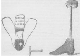
The boot has been most carefully manufactured for me by Messrs. Arnold and Sons, 35, West Smithfield, and is well represented in the diagram. Figure I shews the boot applied; the mechanism at the heel is not noticeable. Figure 2 shews the concealed screw and pinion movement; and the aperture at the heel for the insertion and rotation of the key.
