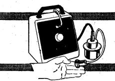
**Plethysmography** Plethysmograph pick-up with three interchangeable digital adaptors.
