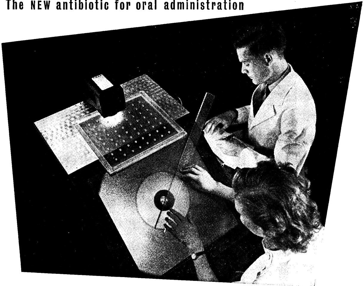
ILLUSTRATION: Evaluation of antibiotic activity by measuring inhibitory zones on agar plates
