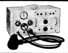
The Pneumotron is an electronically controlled breathing apparatus originally designed for promoting and sustaining breathing in new-born infants, and which has now been developed for treating adult patients. It can be operated as a 'patient triggered' or fully automatic resuscitator. The slightest inspiratory effort of the patient will 'trigger' the apparatus to follow the breathing rate and respiratory pattern of the patient.
