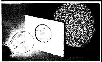
EVEN, ALL-OVER POROSITY Project images of the filament of a clear electric lamp through the pores of stretched Elastoplast on to a white surface. See how even the filament pattern is. Elastoplast leaves no occluded patches of skin even when there is more than one layer.
