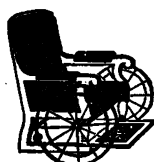
No. 1.—Self-propelling Chair, mounted on 24-in. wheels outside, and may be used by a child eight years of age with the greatest ease.
