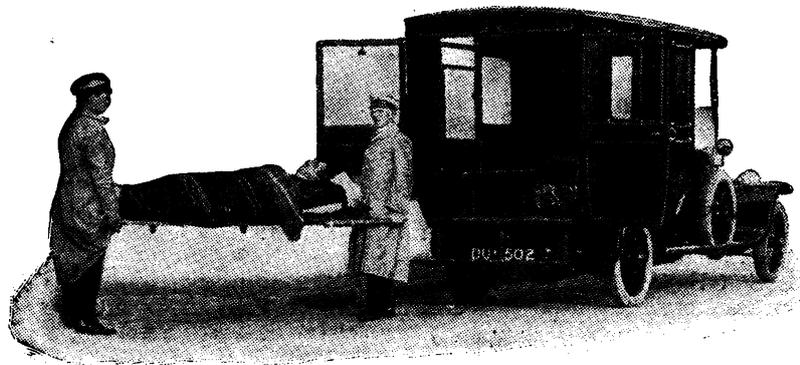
**D**AIMLER Ambulances are fully equipped to afford the utmost comfort to the patient, including Stretcher mounted on special springs, Carrying Chair, Air-Bed, Waterproof Sheeting, Washstand (with an ample supply of water) and a fresh supply of linen for each case.
