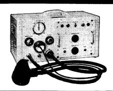
The Pneumotron is an electronically controlled breathing apparatus originally designed for promoting and sustaining breathing in new-born infants, and which has now been developed for treating adult patients. It can be operated as a 'patient triggered' or fully automatic resuscitator. The slightest inspiratory effort of the patient will 'trigger' the apparatus to follow the breathing rate and respiratory pattern of the patient.
