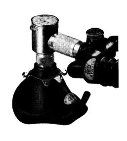
This respiratory measuring instrument for use in anaesthesia, oxygen therapy and for general application in respiratory physiology has a watch-type dial which shows at a glance the precise amount of gas that has passed through the instrument. Air resistance and inertia are extremely low, and the instrument can be plugged into any part of an anaesthetic circuit or used with a face mask for respiratory studies.
